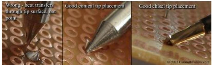
Now melt solder on the opposite side of the lead and pad from where the iron is touching. This will ensure the parts are hot enough to bond with the solder, and will also help to spread the solder over the connection, as it will be drawn to the heat. Remove the solder, then the iron a bit later. Larger components will require more heat and time for the solder to coat the connection. You should be left with a small volcano that smoothly ramps into all the surfaces.
