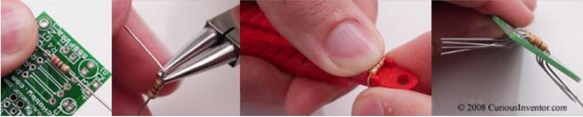
Insert all components as far as possible without excessive force. Bend out the leads to hold the resistor in place while soldering. The resistor codes are: R2: 240 Ohms (Red-Yellow-Brown), R3: 270 (Red-Purple-Brown), R4: 330 (Orange-Orange-Brown), R1: 820 (Grey-Red-Brown). Leave R1 off if you're going to use your own pot to adjust the voltage.
