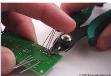
Trim the leads after soldering, safety glasses are a good idea for this. A finger at the end will help contain the shrapnel, but be wary of the thicker leads.
