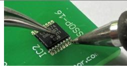
**4)** Check alignment! Once you solder more than one pin, it will be impossible to realign the IC. Reheat the corner pin and nudge the IC into position if it moved off the pads.
