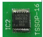
**7)** Use the wick to remove the excess solder. Hold the wick over the pins, and pressure down lightly with the iron. Surface tension will prevent all the solder from wicking off leaving just enough to form a connection.
