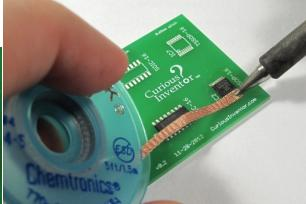
**Be careful #2!** It's very easy to pull pads and pins off with the wick. If a portion of the wick cools while you're moving the wick, it will tear off whatever is frozen to it. Avoid dragging the wick side-to-side to prevent this.
