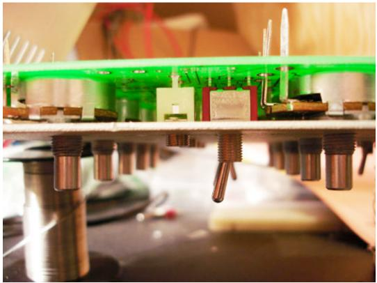
Note the gap between the bottom of the jack and switch and the pcb.
