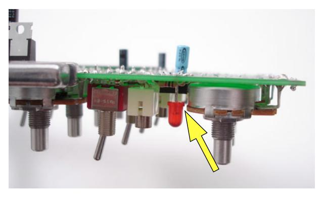
If you look at the top of the LED, you'll notice it's bottom rim forms a D shape. Make sure this aligns with the D shape on the pcb.
