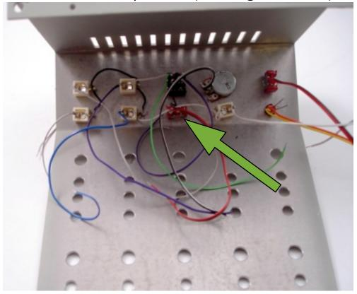
We recommend 14" wires to allow enough room between the pcb and panel for troubleshooting. The green arrow points out the horizontal Clock on/off switch orientation. The other switches are vertical.
