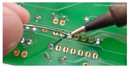
As you are soldering, cut off the leads as you go with flush cutters. Watch out for flying leads; safety glass are actually not over-precatious for this, although we generally just hold the lead with fingers to keep it from flying off.
