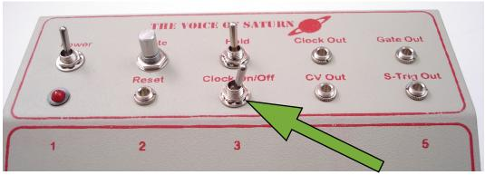
Note the clock switch is installed Left/Right, not up down to accommodate the PCB.
