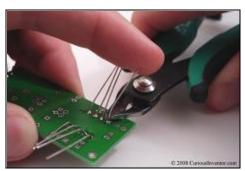
Trim the leads after soldering, safety glasses are a good idea for this. A finger at the end will help contain the shrapnel, but be wary of the thicker leads.
