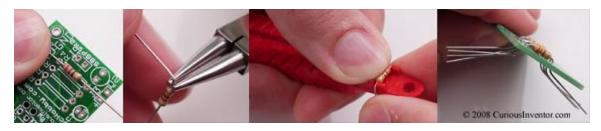
Insert all components as far as possible without excessive force. Bend out the leads to hold the resistor in place while soldering. The resistor codes are: R2: 240 Ohms (Red-Yellow-Brown), R3: 270 (Red-Purple-Brown), R4: 330 (Orange-Orange-Brown), R1: 820 (Grey-Red-Brown). Leave R1 off if you're going to use your own pot to adjust the voltage.
