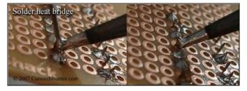
If there isn't enough solder on the iron tip from "tinning the tip," little heat will transfer from it (a "dry" tip). It's important to have a little solder between the iron tip and work. This is called a "**heat bridge**." Melt a small amount of solder between the tip and lead, and then continue adding solder on the opposite side.
