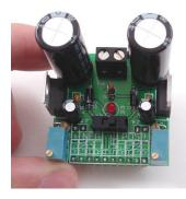
**Install the remaining electrolytic capacitors: C1,C2,C5,C6 (the cylinders).** Be sure to put the longer pin in the positive hole.
