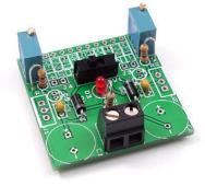
Install P1, RV1 and RV2. The screw on the trim pots should be in the corner.
