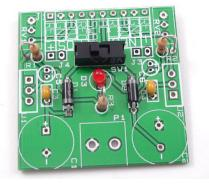
Trim the leads after soldering the components (do this after each step).
